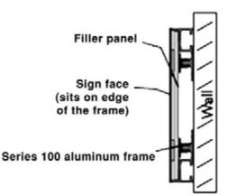
Use the series 100 Framing System for "the frameless look". Cut filler piece of material to fit inside the frame - adhere larger shape to filler piece to hide edges of frame. Use snap locks on filler piece to hold into frame.
