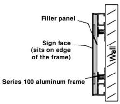
Use the series 100 Framing System for "the frameless look". Cut filler piece of material to fit inside the frame - adhere larger shape to filler piece to hide edges of frame. Use snap locks on filler piece to hold into frame.
